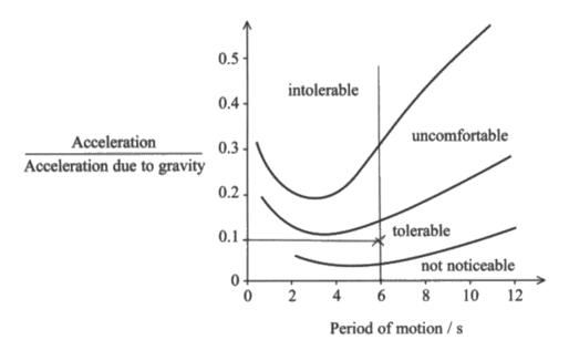
Determine whether the passengers are likely to feel seasick as a result of the ship's motion.
